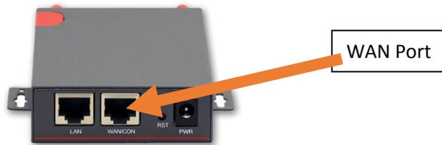
7. Finally, take the Ethernet cable that you connected to the Location switch and connect it to the **LAN** port of the Router.
