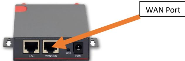
6. Detach the Ethernet cable of the device that you will back up from the Switch. **This will result in an interruption in internet service for the device you have chosen. It will resume once you have successfully installed the Router.**
